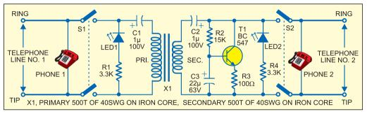
cuit is built around transistor T1 (BC547), resistors R2 and R3 (15 kiloohms and 100 ohms, respectively), condenser C3 ( $22\mu$ F, 63V) and two LEDs as indicators for both the primary and secondary sides. It provides proper DC characteristic to hold second telephone of the circuit is provided by condenser C3, which prevents any audio signal from appearing at the base of T1. Thus any audio voltage appearing across telephone line No. 2 will not cause a corresponding current in the transistor.
